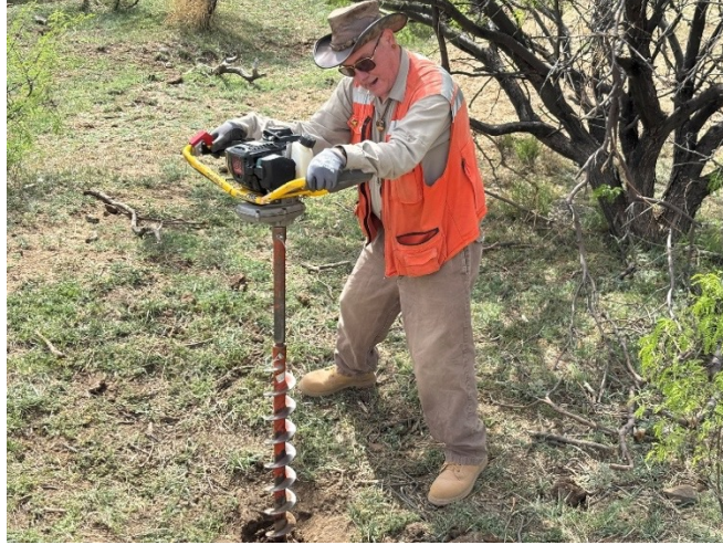
Figure 3: Allan Using Auger to Collect a Samples at One of the Tailings ponds
